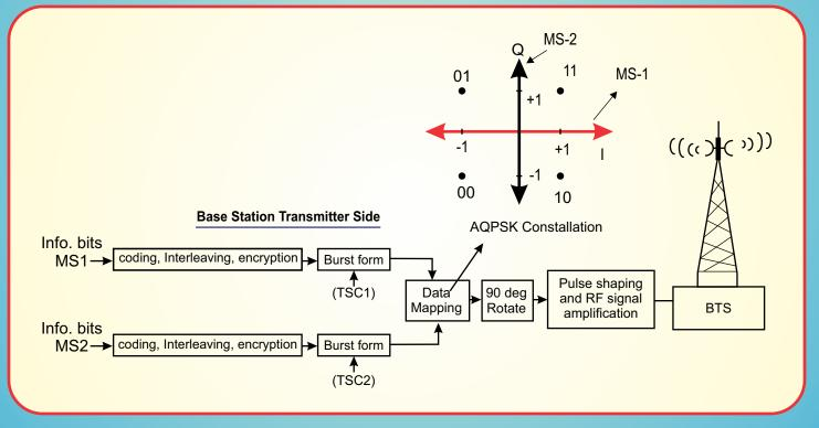
VAMOS Modules for transmissions to two mobile stations MS1 and MS2
