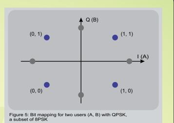
User A is mapped to the first bit and user B to the second bit, with the resulting signals appearing along the 'I' or 'Q' axis, respectively. QPSK is switched to GMSK when only one sub channel is active to also facilitate DTX gains. The transmitter switches off when both sub channels are inactive. Switching from QPSK to GMSK is possible to make signaling more robust. This switching between modulations is transparent to the legacy SAIC handset because it expects to receive GMSK all the time.
